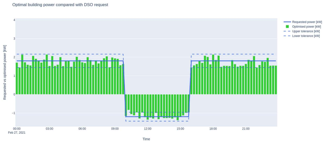
Figure 74 Optimal building power demand to maintain the building and DHW temperatures at desired setpoints (20 °C and 48 °C) and fulfilling at the same time the provisioning of flexibility services to the grid (winter)
