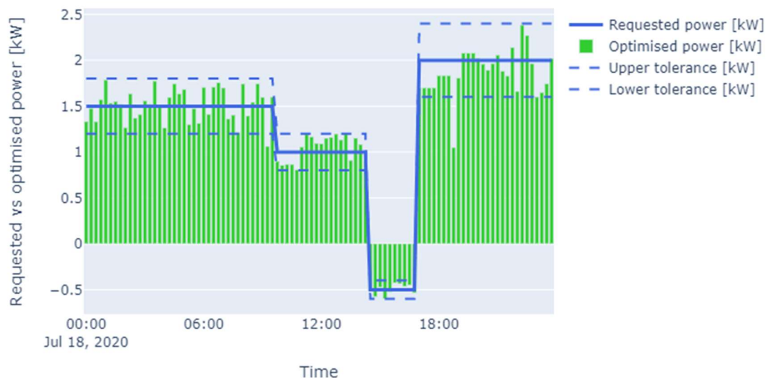
Figure 71 Optimal building power demand to maintain the building and DHW temperatures at desired setpoints (25 °C and 48 °C) and fulfilling at the same time the provisioning of flexibility services to the grid (summer)
