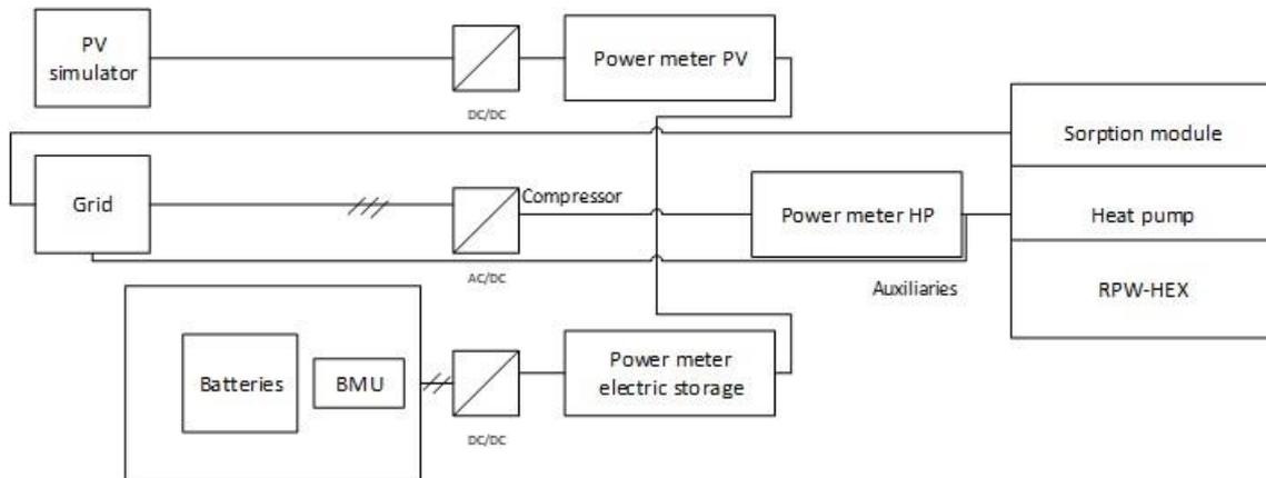
Figure 2: Mediterranean system integrated in the lab - detail of electric connections.
