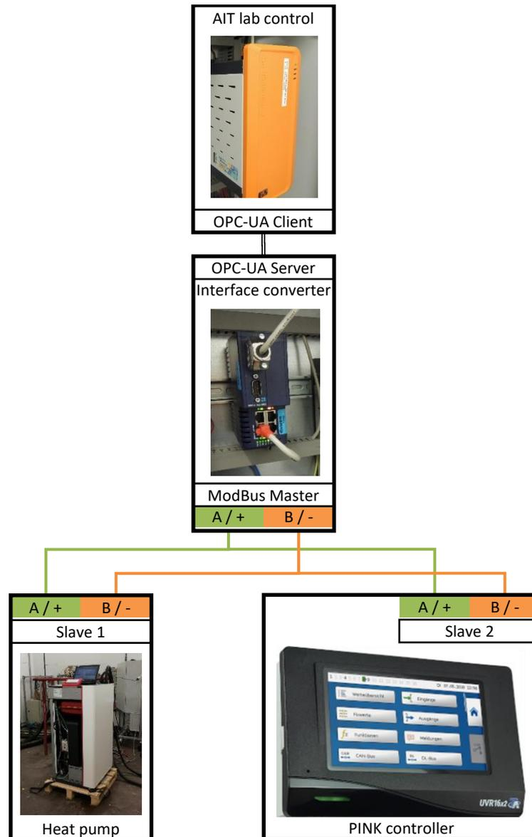
Figure 39: Schema of the connection between the individual controllers
