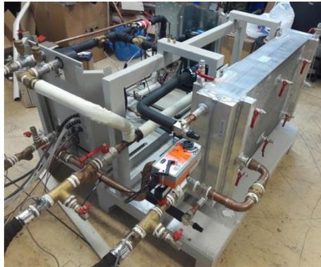
Figure 5 The retrofitted heat pump along with the RPW-HEX
