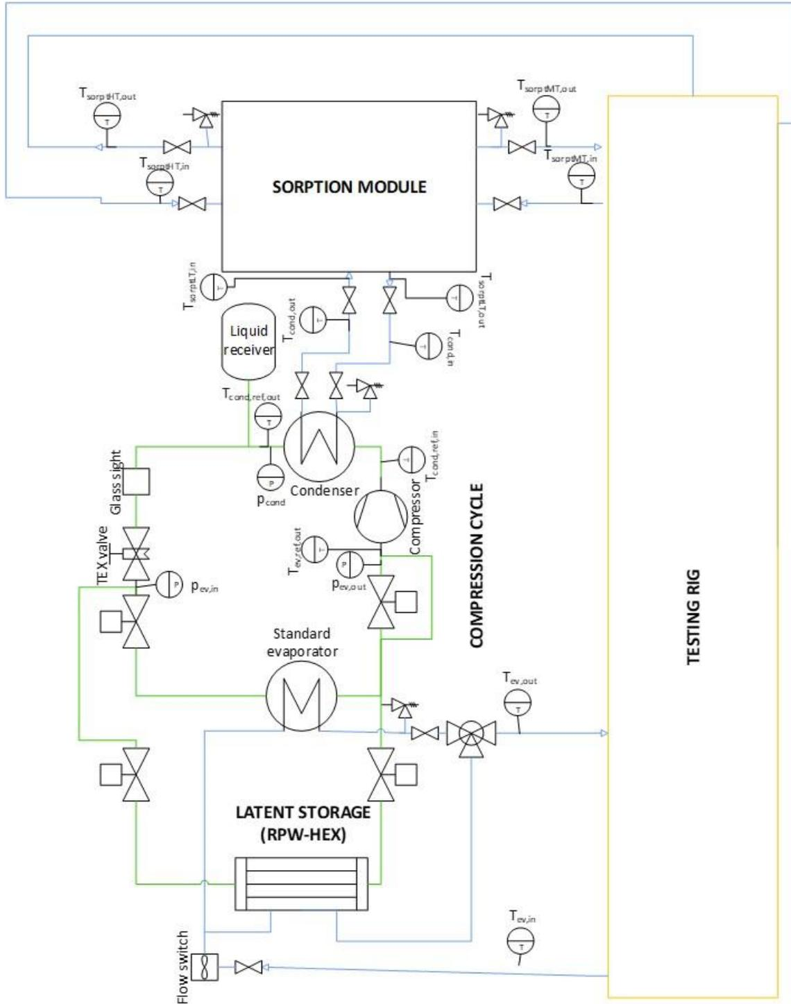
Figure 1: P&ID of Mediterranean subsystem integrated in the lab.
