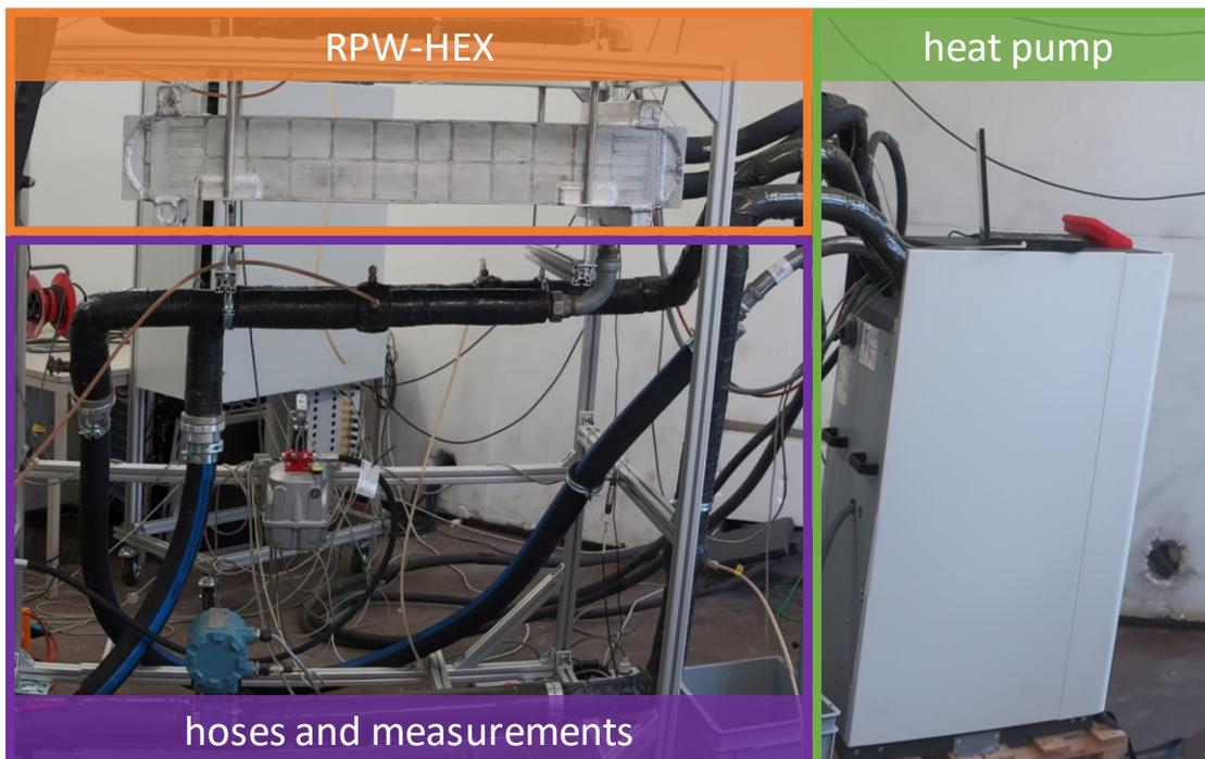
Figure 25: Experimental setup showing the heat pump indoor-unit (green), the RPW-HEX (orange) and hoses and flow measurement sensors (violet).
