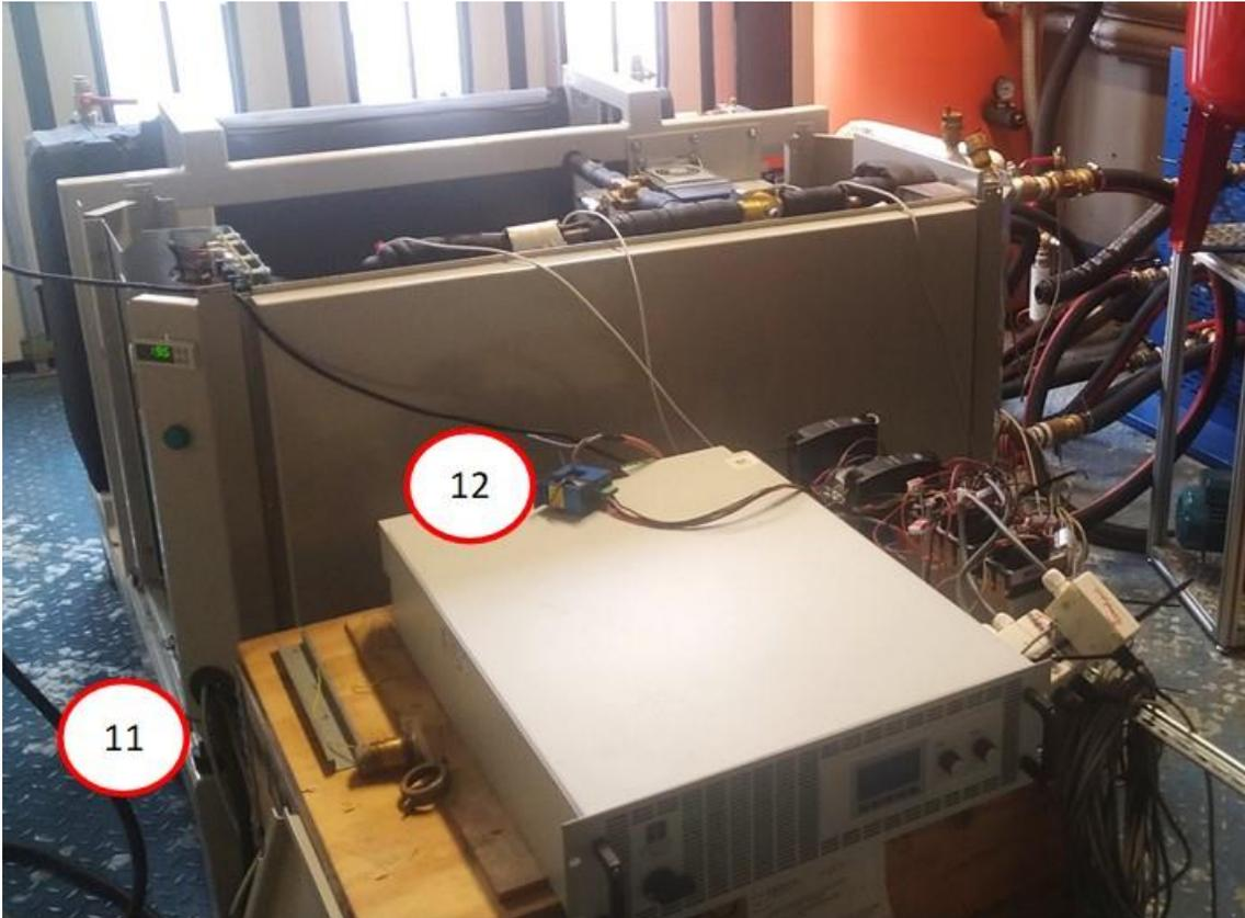
Figure 14: integration of the latent thermal storage in the heat pump – focus on electric connections. 11: cable for DC operation of the heat pump, 12: supply voltage
