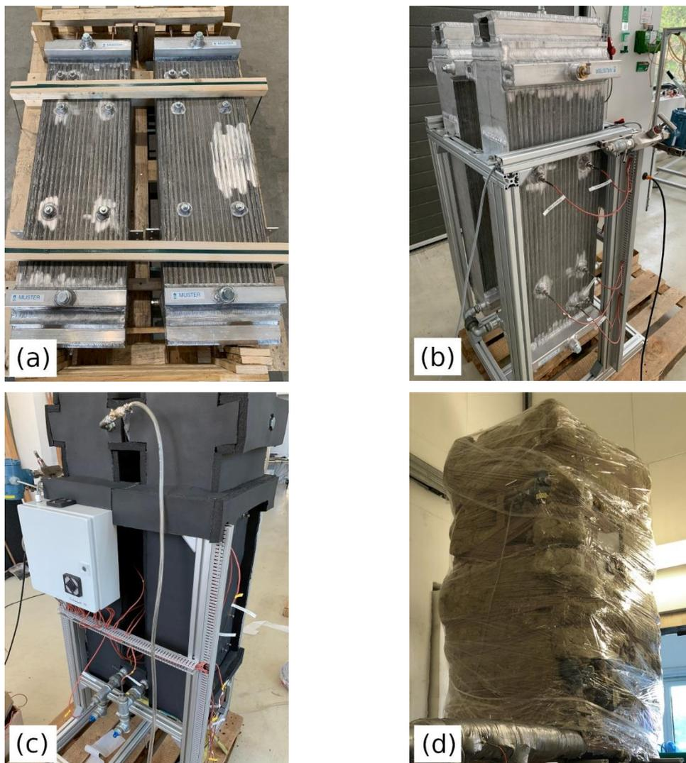
Figure 37: (a) RPW-HEX without insulation and sensors, (b) RPW-HEX equipped with sensors and assembled to the upper part of the supporting frame, (c) RPW-HEX insulated with 3.6 cm Armaflex HT, (d) RPW-HEX integrated in the full set up and insulated with further 10 cm mineral wool.
