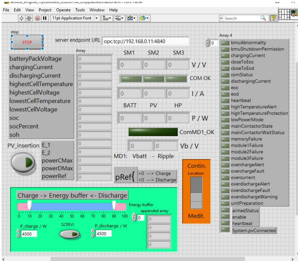
Figure 21: LabVIEW software for testing the OPC-UA communication with the PLC.
