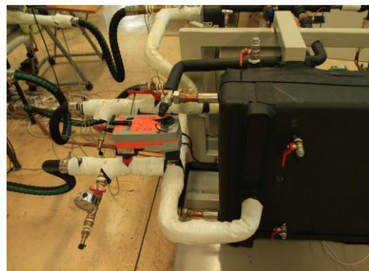
Figure 11 The 3-way ball valve in the evaporator circuit
