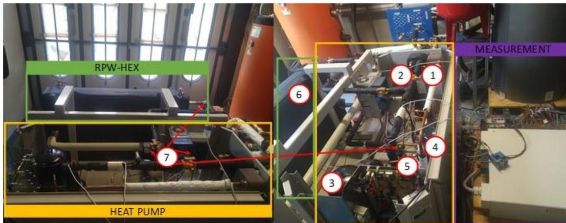
Figure 1: integration of the latent thermal storage in the heat pump – focus on refrigerant circuit. 1: condenser, 2: standard evaporator, 3: compressor, 4: liquid receiver, 5: expansion valve, 6: RPW-HEX
