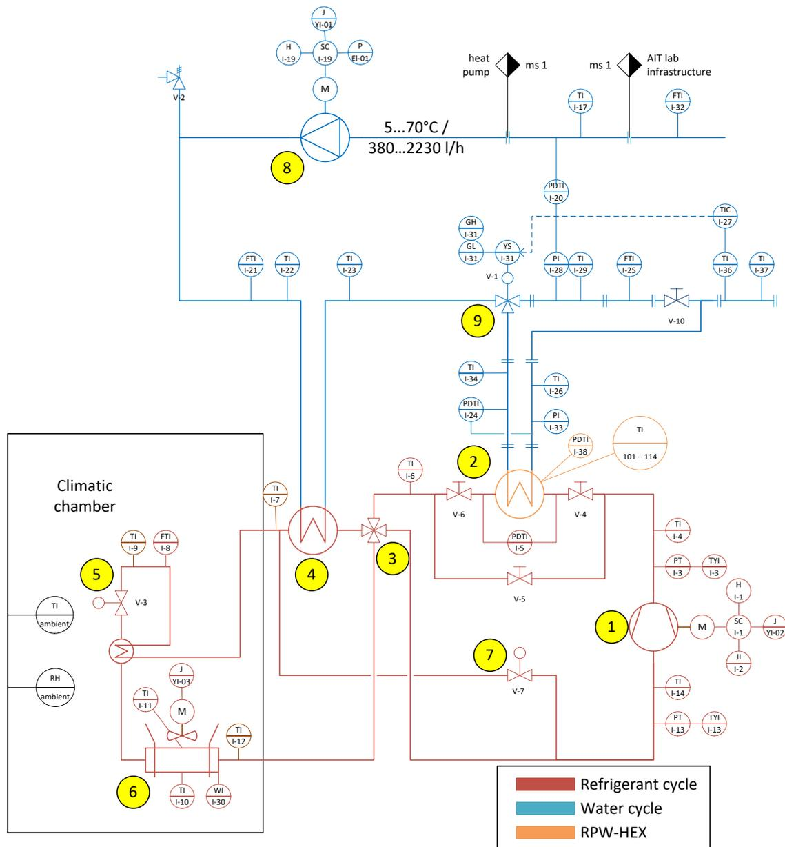
Figure 23: P&ID of the experimental setup to perform tests with RPW-HEX Version 1. ① Compressor, ② thermal storage (RPW-HEX), ③ 4-way-valve, ④ Condenser, ⑤ Expansion valve, ⑥ Evaporator, ⑦ Liquid injection valve, ⑧ water pump, ⑨ 3-way-valve. (TI) Temperature sensors, (PT) Pressure sensors, (FTI) mass flow sensors, (SC) speed monitoring, (JI) electric power measurement, (WI) scale.
