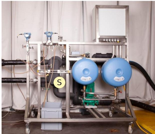
Figure 31: Interface to the AIT lab infrastructure. (S) Plate type heat exchanger working as a heat- sink/source for the building water cycle. The other components on the test rig (pumps, controllers, etc.) were not used during the experiments.
