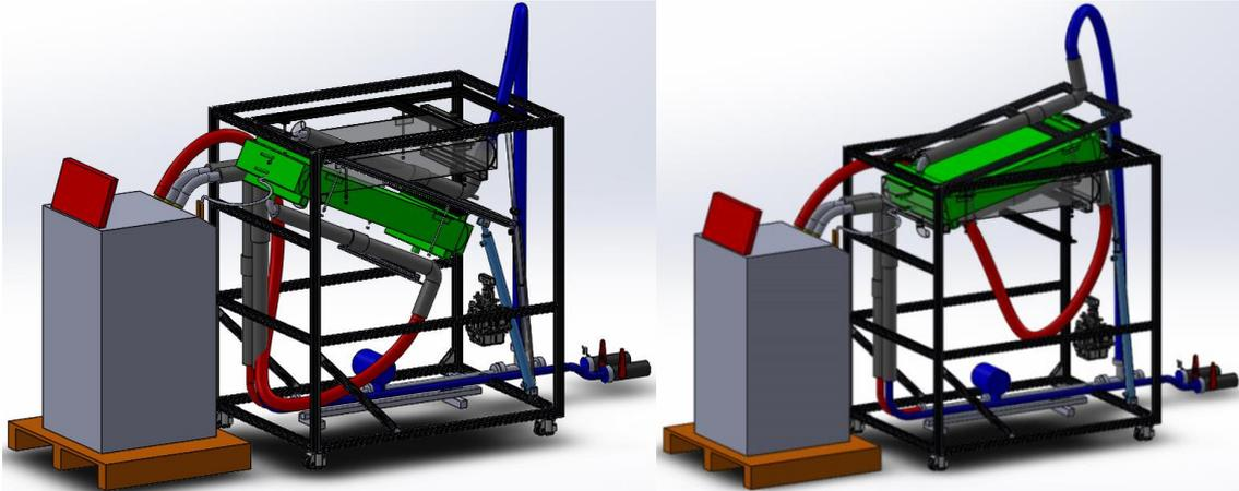
Figure 26: Isometric of the HP with the RPW-HEX mounted onto the special scaffolding. Left: RPW-HEX is tilted down. Right: RPW-HEX is tilted up.
