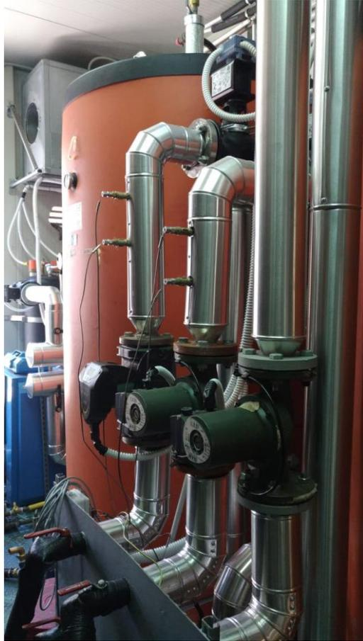
Figure 16: sensors in the testing rig for the sorption module characterization.
