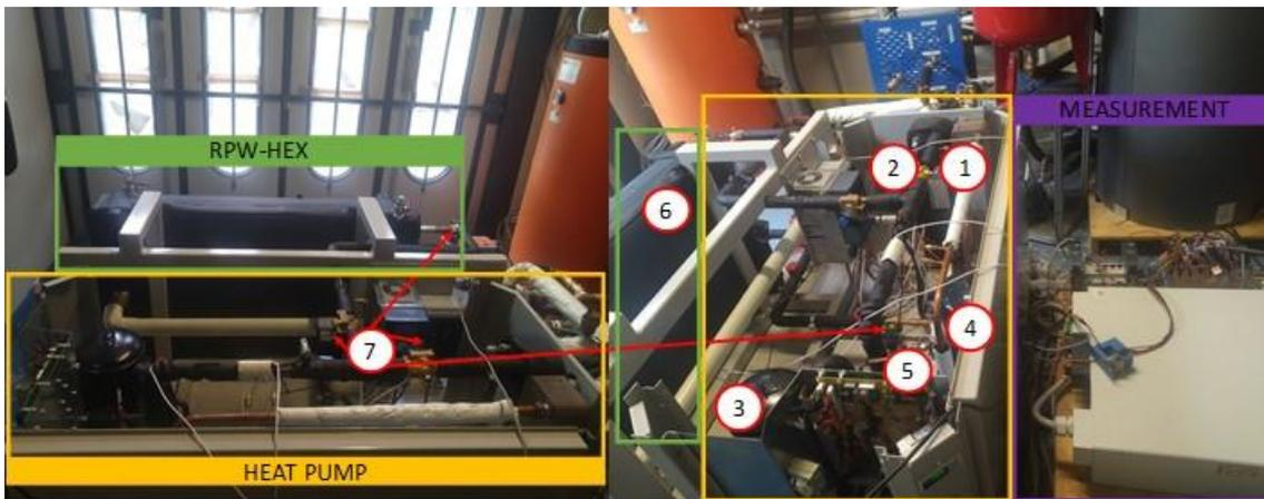
Figure 6: integration of the latent thermal storage in the heat pump – focus on refrigerant circuit. 1: condenser, 2: standard evaporator, 3: compressor, 4: liquid receiver, 5: expansion valve, 6: RPW-HEX
