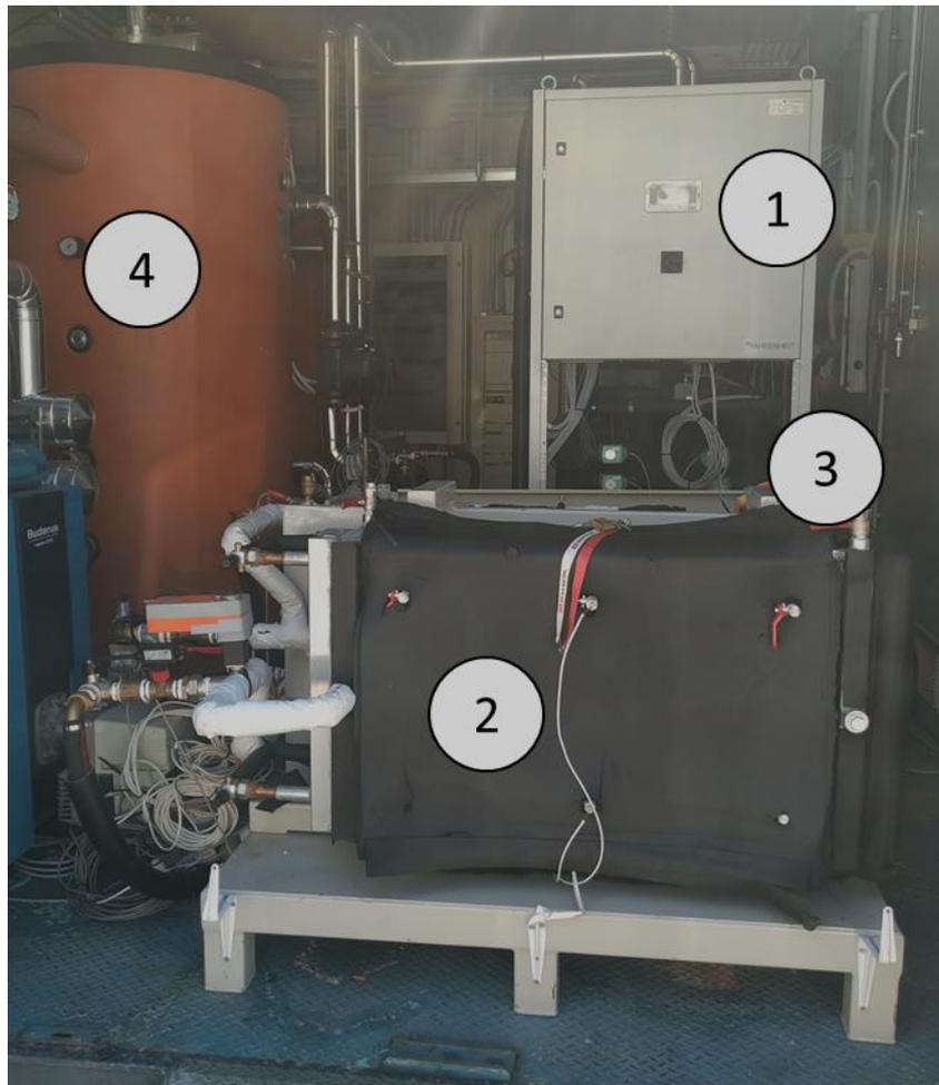
Figure 3: MED sub-system in the lab of ITAE. 1: sorption module; 2: heat pump with RPW-HEX; 3: electric connection to the rack; 4: testing rig.
