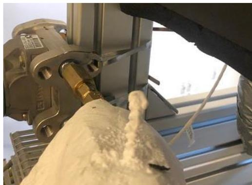
Figure 40: Accumulation of PCM below a leaking connection
