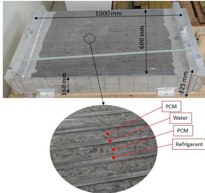
Figure 24: Picture of the RPW-HEX with external dimensions and detailed view of the micro channels.
