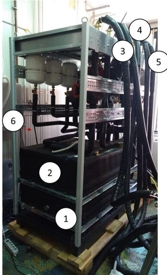
Figure 15: sorption module integrated with heat pump. 1, 2: adsorbers and evaporators/condensers; 3: pipes of LT circuit; 4: pipes of MT circuit; 5: pipes of HT circuit; 6: cable for supply voltage.
