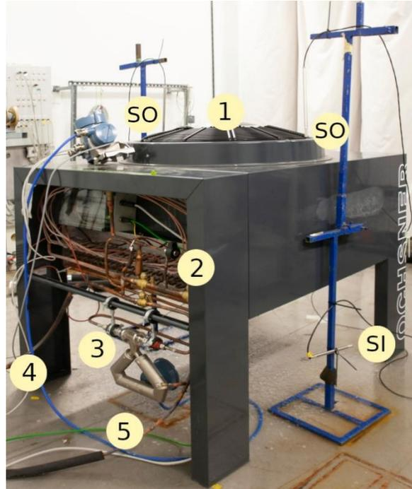
**Figure 38: Outdoor unit of the air-source heat pump located in the outdoor climatic chamber. (1) fan, (2) evaporator mounted horizontally below the fan, (3) Coriolis mass flow meter (FT18), (4) and (5) refrigerant line from and to the indoor unit, respectively, (SI) and (SO) temperature and moisture sensors close to the air inlet and outlet, respectively.**
