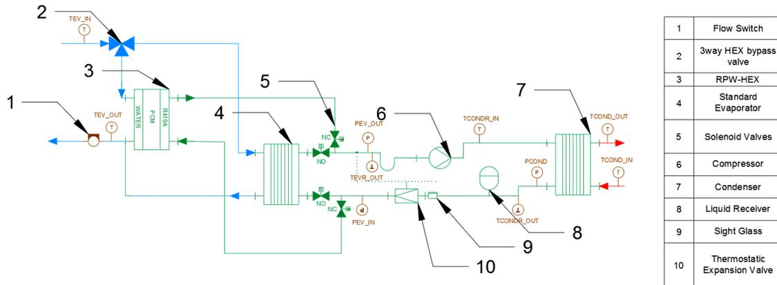
**Figure 4: Schematic diagram of the compression heat pump setup in lab for the Mediterranean concept (installed sensors marked in red)**
