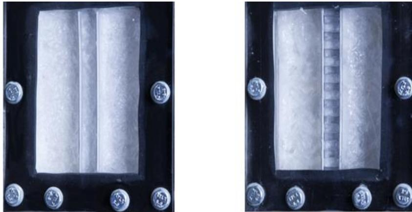
Figure 22: PCM-samples filled with RT64HC with no fins (left) and straight fins (right) and 1 cm distance between MPE-tubes.
