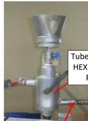
Tube-in-tube HEX to melt PCM
