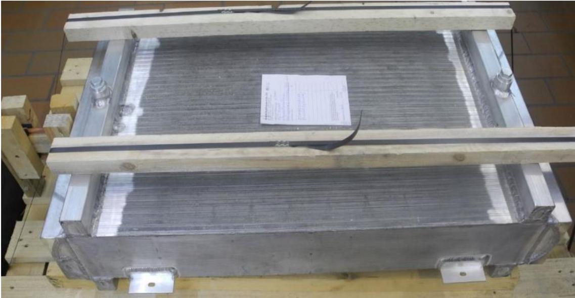
Figure 58. Photo of high temperature full-scale latent storage for AIT (NP 4012812)
