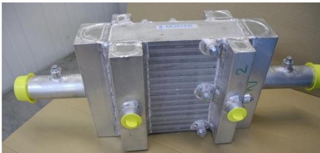
Subsequently, several small-scale RPW-HEXs were manufactured by AKG and shipped to UDL and AIT for lab testing. Heat transfer and pressure drops in several designs were calculated by using literature or specific equations developed by AKG and used to optimise the lab-scale storages manufactured. The
