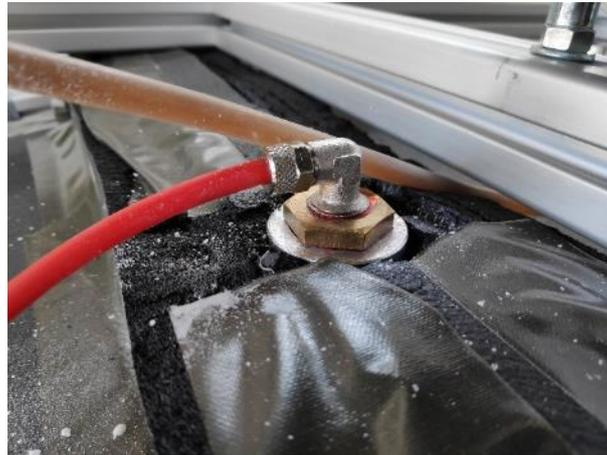
Figure 69: RPW-HEX PCM pressure measurement.
