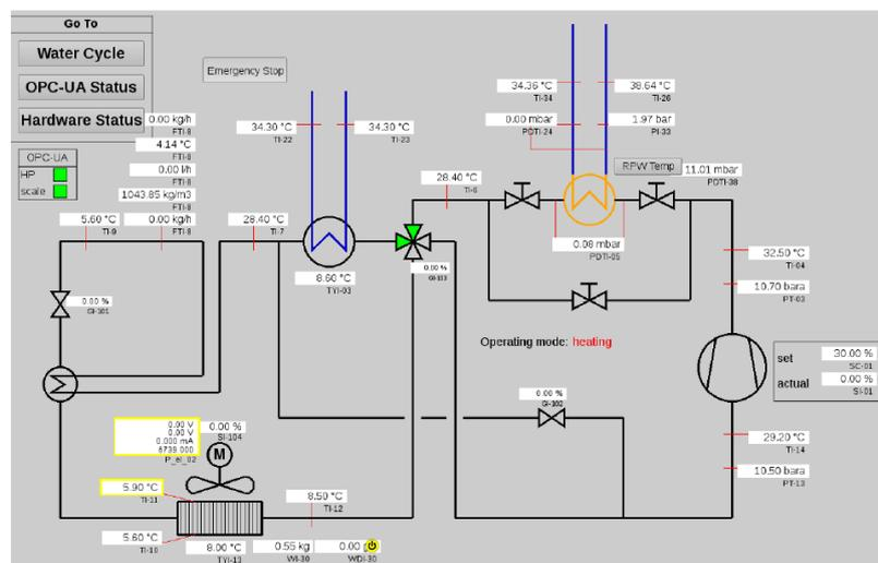
Figure 28: Screenshot of the APROL DISPLAY CENTER showing all the sensors and their current values in the refrigerant cycle.
