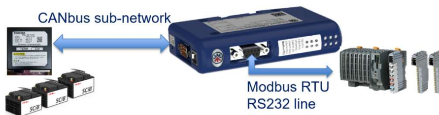
Figure 17 - Schematic representation of the data exchange architecture from PCS (Modbus RTU) to BMU (proprietary CANbus) and viceversa, through a conversion gateway
