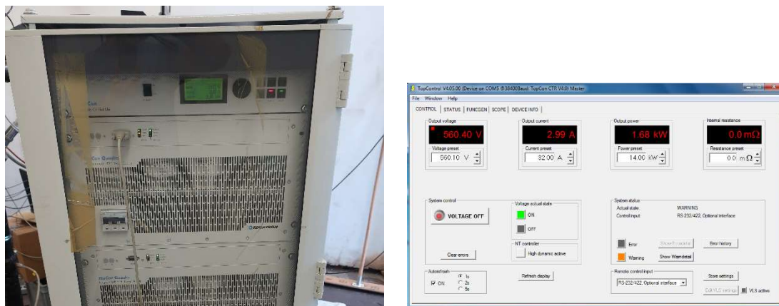
Figure 18 DC bus generator (left) and software interface (right).
