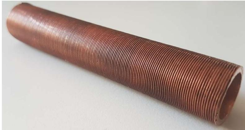
Figure 81: Sample for finned copper tubes
