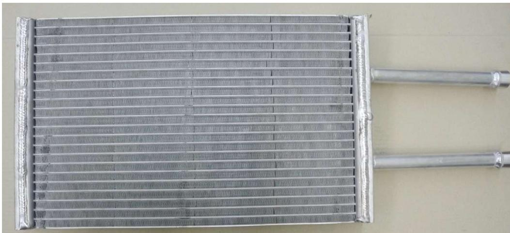
Figure 41: Photo of medium-size adsorber (NP: 4013590)
