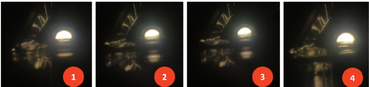
Figure 77: Process of bubble formation and collapsing for 45° arrangement.
