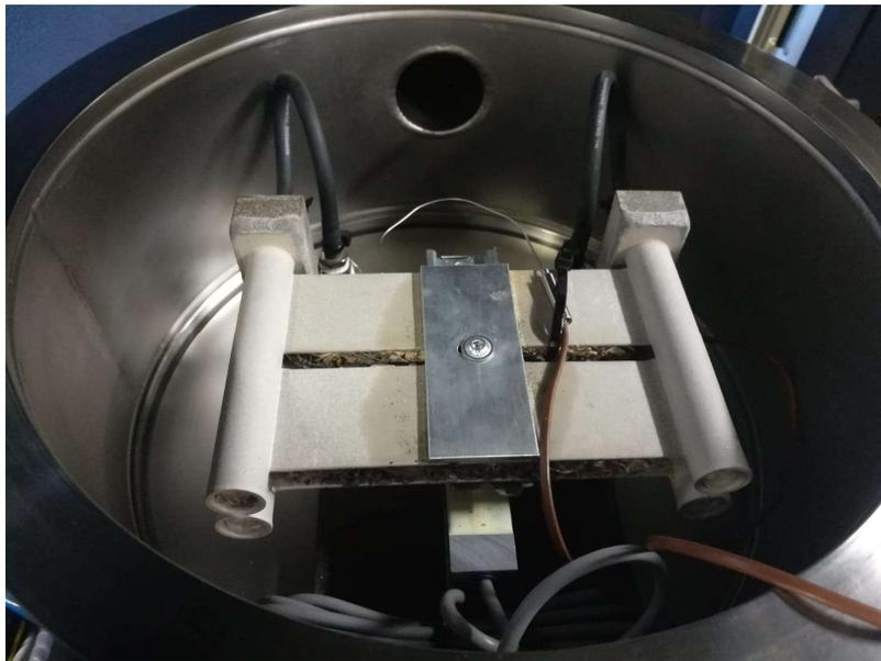
Figure 27: View of the adsorber installed in the measuring unit.
