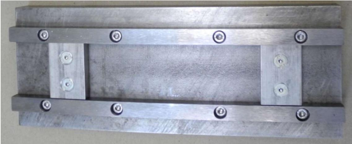
Figure 37: Gauge for checking and calibrating the compressed fins
