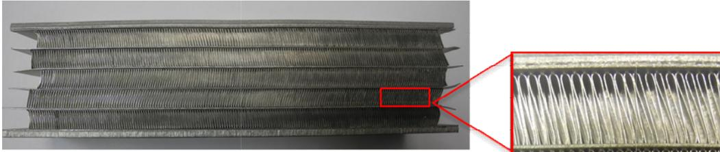
Figure 44: Evaporator demonstrator with dense fins and MPE-tubes
