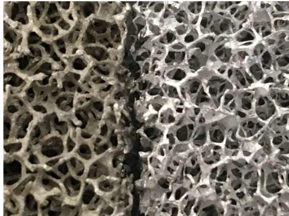
Figure 15: Wire thickness before and after crystallization process of non-useful foam sample
