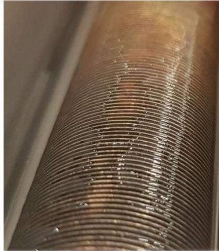
Figure 83: Capillary effect for good heat transfer without big surface areas
